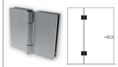
Maximum door width = 900mm Maximum door weight = 50Kgs Glass thickness = 8mm - 12mm
