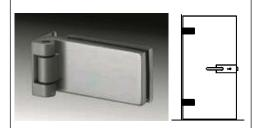
Maximum door width = 1000mm Maximum door weight = 50Kgs Glass thickness = 8mm - 12mm Torque Setting = 14-16 Nm
