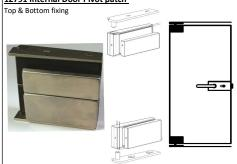
Maximum door width = 1000mm Maximum door weight = 60Kgs Glass thickness = 8mm - 12mm Torque Setting = 14-16 Nm
